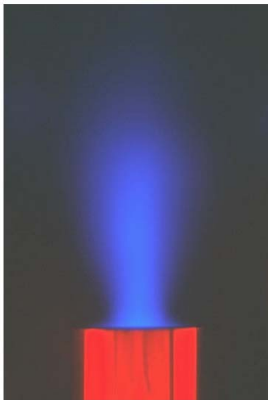
Fig. 2. Sonoluminescence produced in a liquid under ultrasound excitation.
