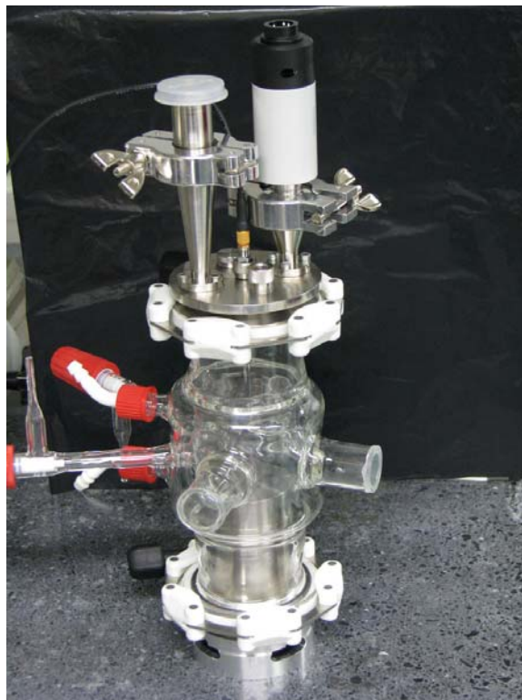
The sonochemical cell allowing spectroscopy of photoluminescence linked to cavitation and simultaneous control of solutes and gas
