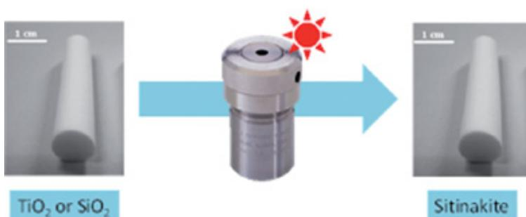
Figure 2: Pseudomorphous transformation general principle used to prepare sitinakite monolithic materials
