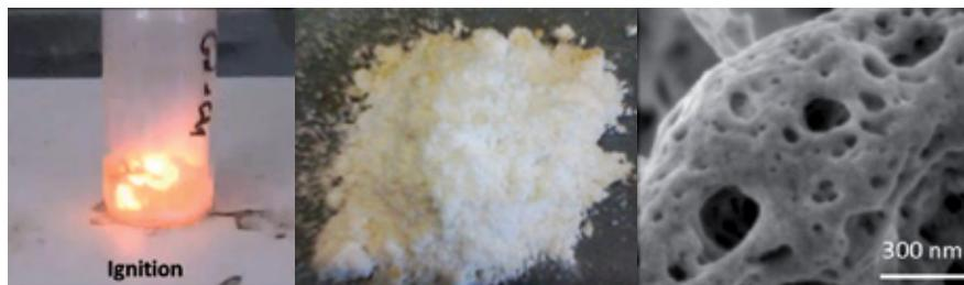
Figure 1 : Example of actinide surrogate powders  $\text{Gd}_2\text{O}_3$  obtained by SCS of Gadolinium nitrate/Glycine
