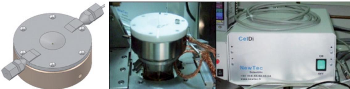
Fig. 1: Artist view of the CelDi tool and pictures of the tool that has been built.
