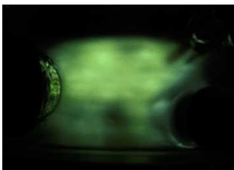
Figure 1: Photograph of 0.031\text{M UO}_2^{2+} sonoluminescence in 0.5\text{M H}_3\text{PO}_4 at 203\text{kHz} under argon flow, LP = 63\text{W} , T = 10^\circ\text{C} , exposure time 30 sec, and sonoluminescence spectra of 0.5\text{M H}_3\text{PO}_4 and 0.05\text{M UO}_2^{2+} in 0.5\text{M H}_3\text{PO}_4 at 203\text{kHz} , LP = 61\text{W} , T = 10^\circ\text{C} , Ar.
