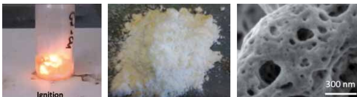
Figure 1 : Example of actinide surrogate powders \text{Gd}_2\text{O}_3 obtained by SCS of Gadolinium nitrate/Glycine
