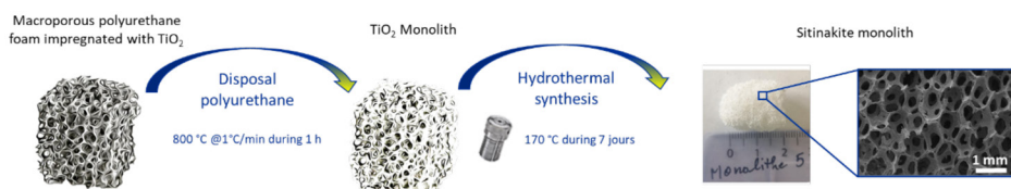
Figure 2. Pseudomorphic transformation of \text{TiO}_2 monoliths into sitinakite.
